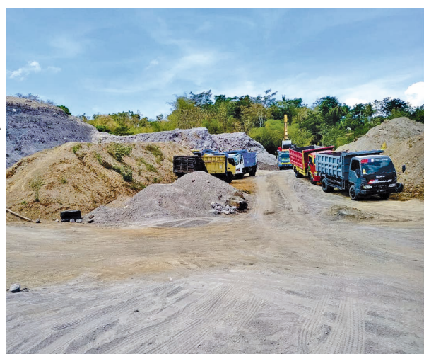
Loading sirtu (sandstone) by Elf Truck with a capacity of 6 m 3
